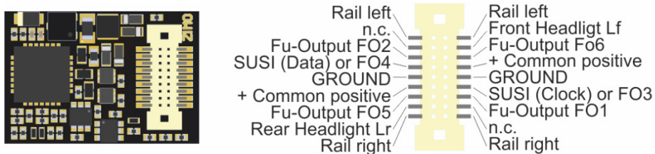
Connection diagram MX689N18 Plug Side View (Next-18)
