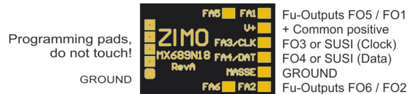
Connection diagram MX689N18 Bottom Side View (Next-18)
